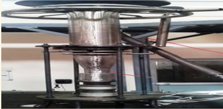
Fig. 1: Duct Mounted 42 GHz, 200 kW Gyrotron
