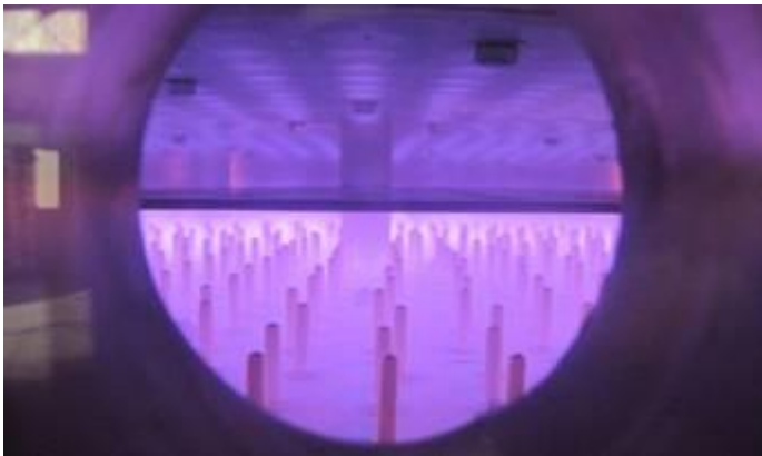
Plasma Treatment of Brass Valves
