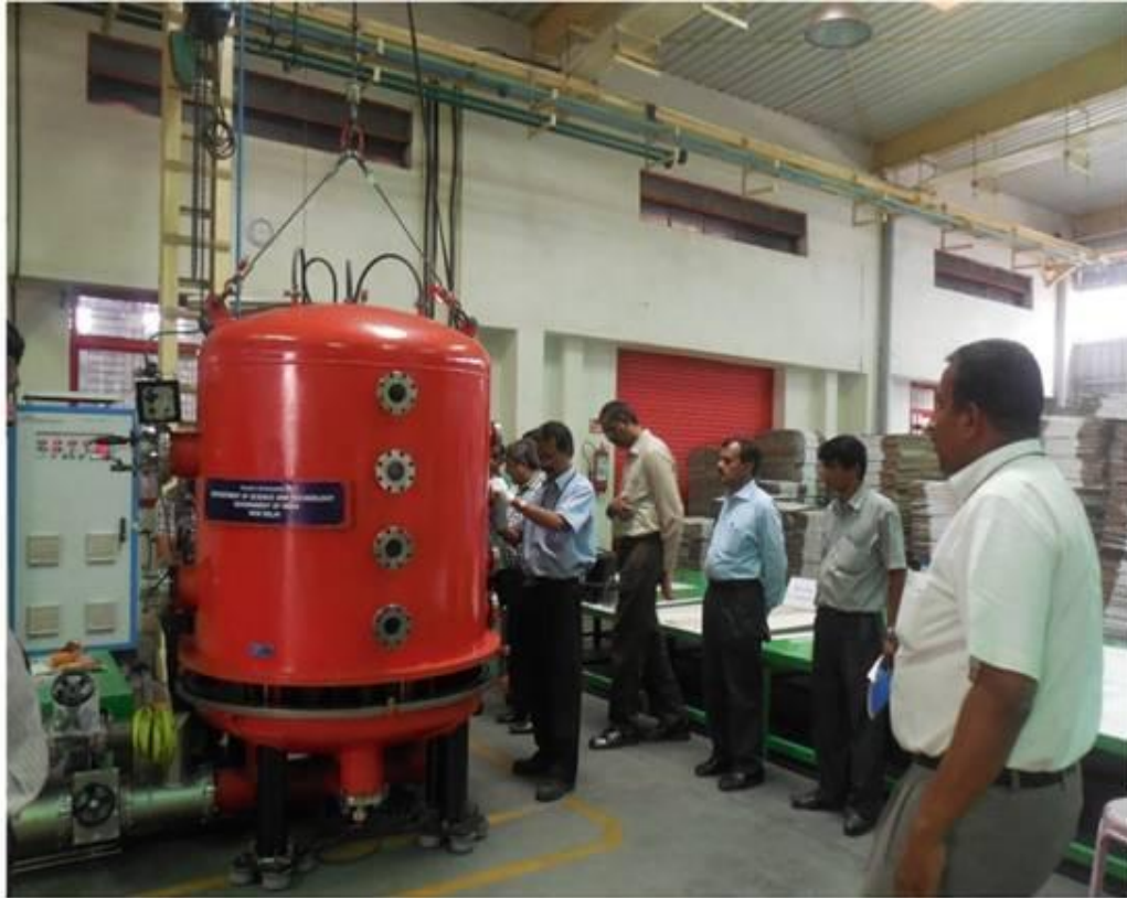
Plasma Treatment System to Treat Brass Valves at M/s. Triton Valves Ltd., Mysore
