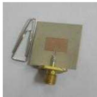
Fig. 2 Miniaturized patch antenna fabricated using high dielectric MW substrates
