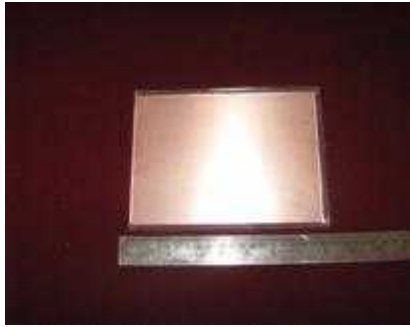
Fig. 3 Band pass filter fabricated using indigenously developed MW substrates
