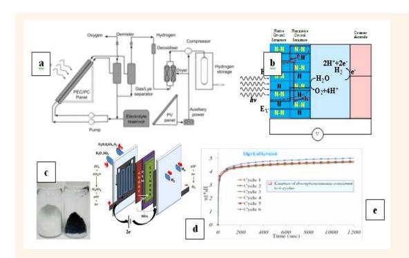
R & D output at multiple-length scales: (a) Solar-H2 process flowsheet; (b) Material design involving native/non-native heterostructures to promote electron-hole separation; (c) Functionalization of material to make a "white" transition metal oxide to "black" thereby increasing the photon absorption cross-section; (d) Sulphuric acid electrolyzer; and (e) Hybrid-organic-metallic alloy for H2 storage.
