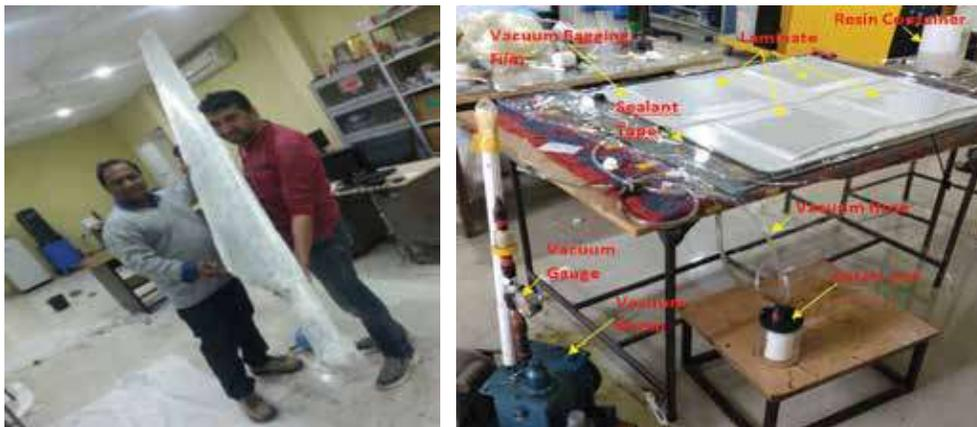
**In-house developed VARTM setup In-house developed wind turbine blade**
