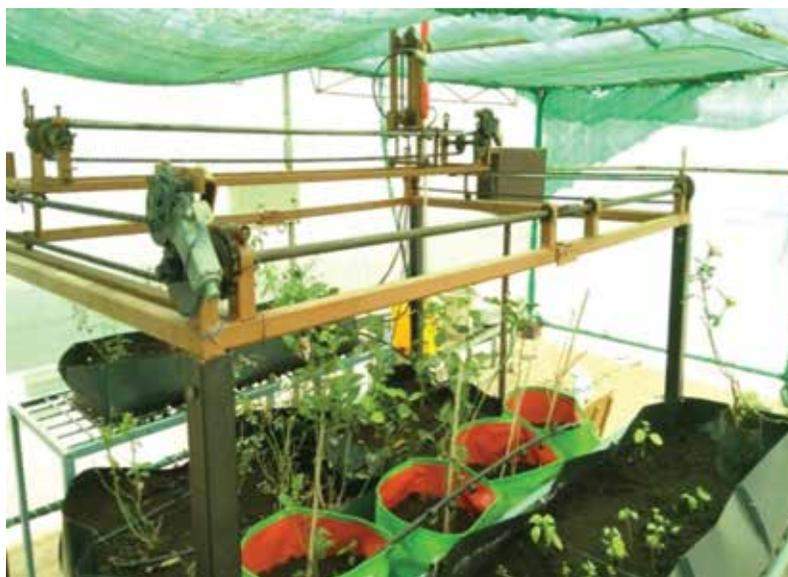
**Fig. Automatic fertilizer supply system**
