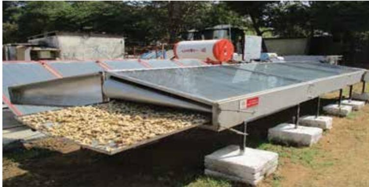
**PV integrated solar dryer installed at Aromatic and Medicinal Research Centre, Anand**
