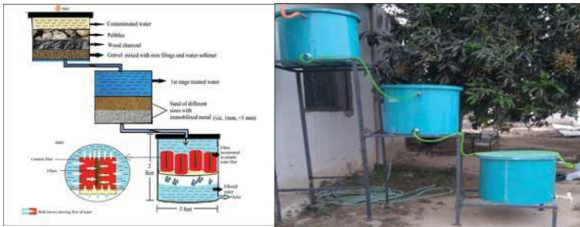
Schematic diagram of the integrated water filter system
