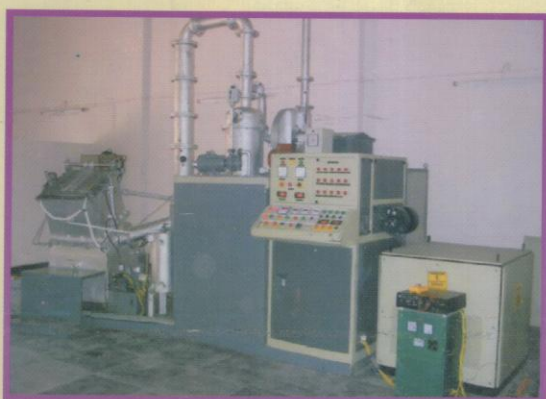
Plasma Waste Destruction System for Plastic and Medical Waste (FCIPT-IPR, Gandhinagar)
