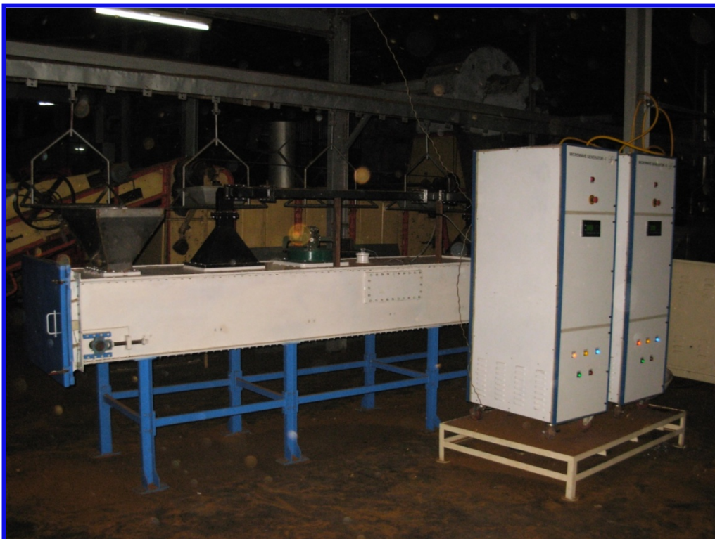
Photograph of field trials of the Variable Power 10 kW Microwave System for Tea Drying at Luxmi Tea Estate, Narayanpur, Assam
