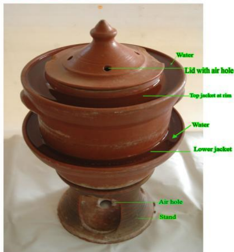
Fig.2.5. Modified earthenware storage system (EWSS-2)
