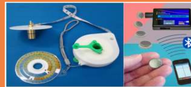
A secchi disk with temperature sensors to be distributed to public as part of citizen science
