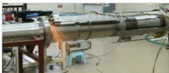
Laser Cutting for Bellow Lip
