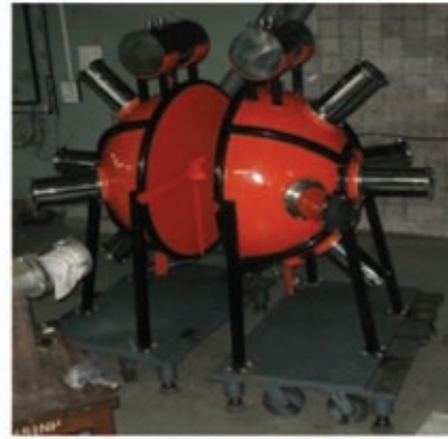
4 \pi Neutron Multiplicity Detector
