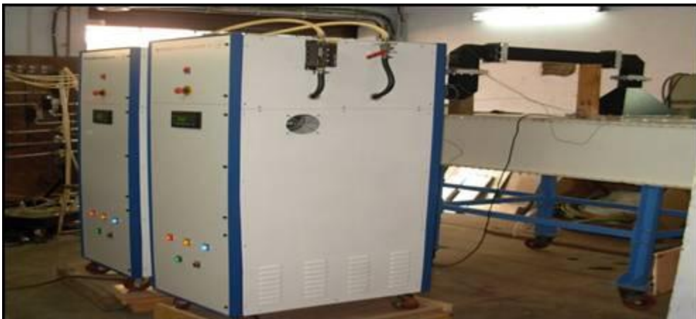
Schematic Diagram of the Variable Power 10 kW Microwave System for Tea Drying
