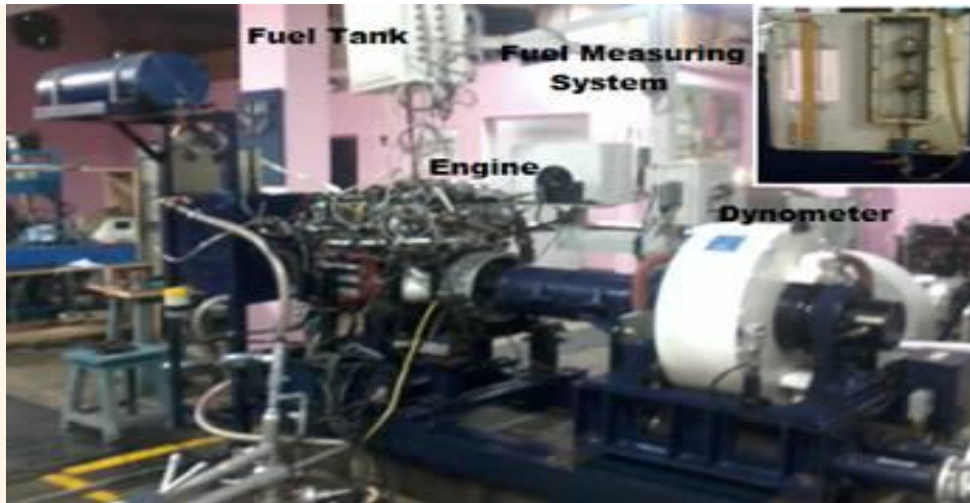
Figure 1: CRDI Diesel Engine coupled with Eddy Current Dynamometer and Controller
