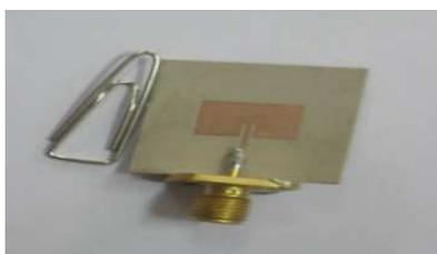
Miniaturized patch antenna fabricated using high dielectric MW substrates
