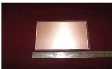
8"x8" size Cu-cladded microwave substrates developed at C-MET through DST funding
