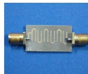
Band pass filter fabricated using indigenously developed MW substrates
