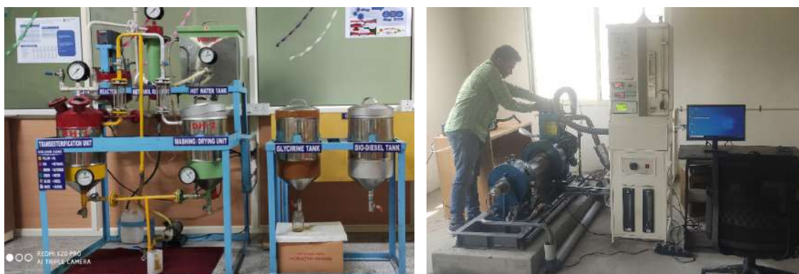
Figure: (a) Biodiesel reactor (10 L per day capacity) and (b) Computerized diesel engine with gas analyser
