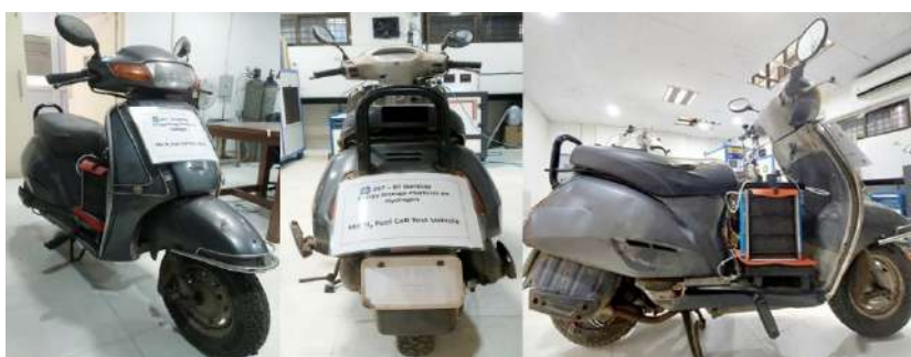
Figure: Proof of concept of metal hydride-based hydrogen storage with PEMFC integrated on a Scooter
