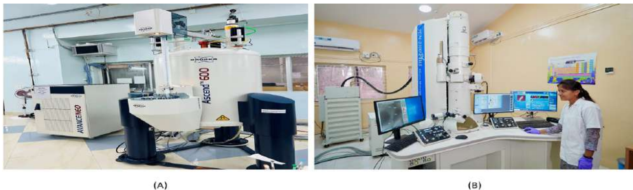
Figure: (A) 600MHz NMR at SAIF Centre at IISc Bangalore and (B) HR-TEM at SAIF Centre at Shivaji University Kolhapur
