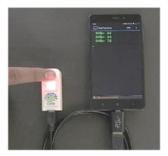
Prof. G U Kulkarni and his co-workers from CeNS, an autonomous institute of the Department of Science and Technology (DST) have fabricated an ultrafast humidity sensor with response and recovery time of around 10-20 milliseconds and successfully integrated into a small stand-alone pen-drive size device which can efficiently sense the breath pattern.
