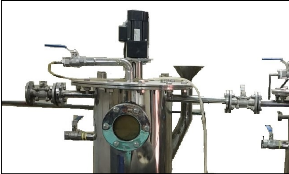
Laboratory scale anaerobic reactor - 45 litre capacity
