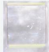
Electronic grade diamond containing single NV defects
