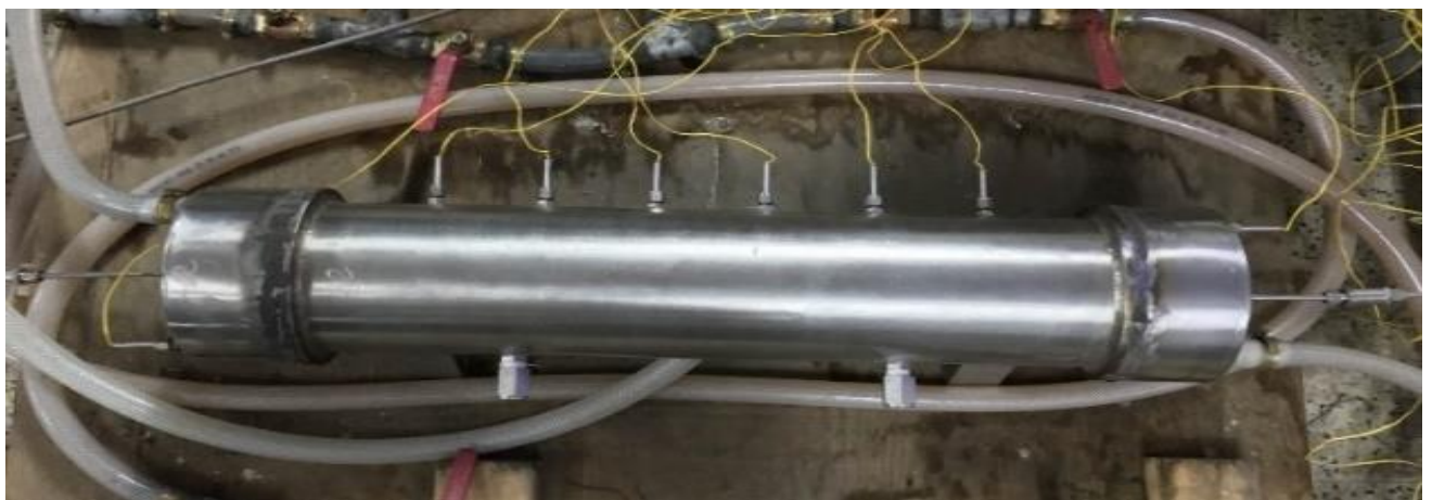
Figure 28. Metal hydride based hydrogen purification system of 1 kg H_2 (99.99% purity) developed at IIT Guwahati
