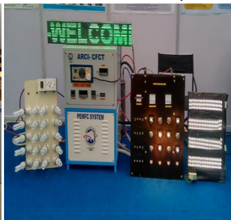
Figure 31. Demonstration of PEMFC system of 3 kW and 5 kW
