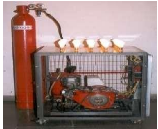
Figure 21. Total hydrogen S.I. engine genset using electronic fuel injection system
