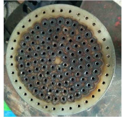
Figure 26. Metal hydride based hydrogen storage system with 4000 liters of hydrogen storage (at STP) capacity developed at IIT Guwahati
