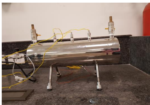
Figure 30. Metal hydride based reactors designed for backup power application with capacity 1.5 kWh and 10kWh resp. developed at IIT Bombay
