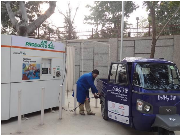
Figure 20. Hydrogen fuelled 3-wheeler developed jointly by IIT Delhi and Mahindra & Mahindra in New Delhi
