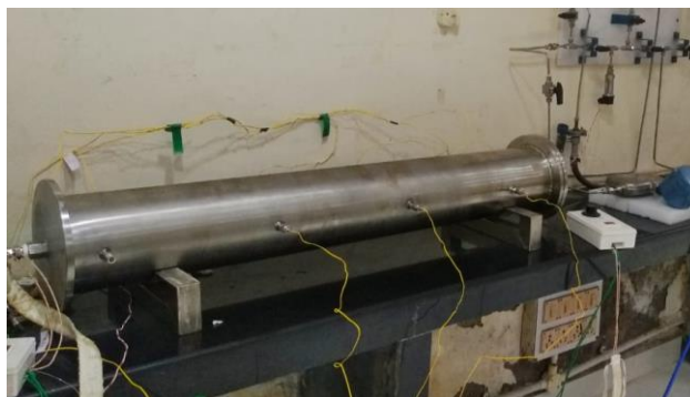
Figure 30. Metal hydride based reactors designed for backup power application with capacity 1.5 kWh and 10kWh resp. developed at IIT Bombay
