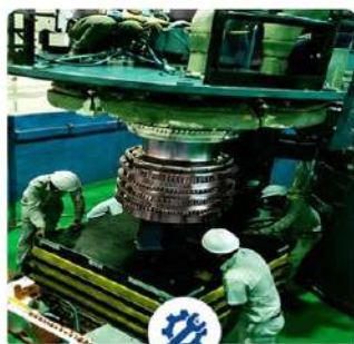
Loading of Mono metallic (Al617) Test Rotor in HTSTR
