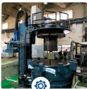
Loading of Mono metallic (Al617) Test Rotor in HTSTR
