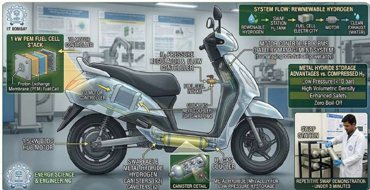
Hydrogen-Powered Scooter Integrated with a Metal Hydride Storage System Demonstrated at IIT Bombay
