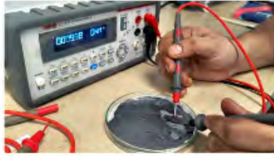
Resistivity of graphene ink coated on filter paper
