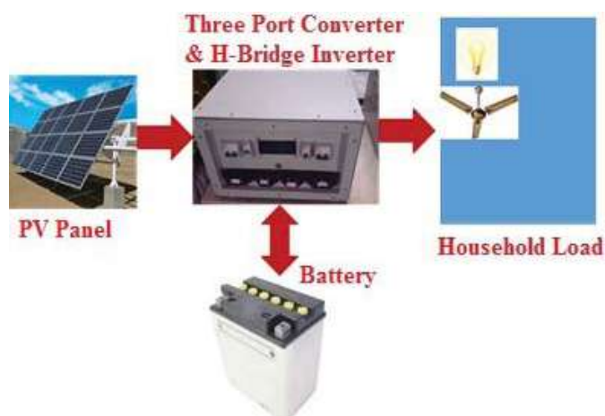
Overview of the proposed scheme of the PV based standalone system
