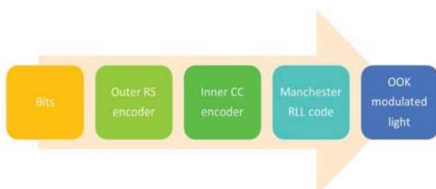
Sample OOK transmitter block diagram for VLC
