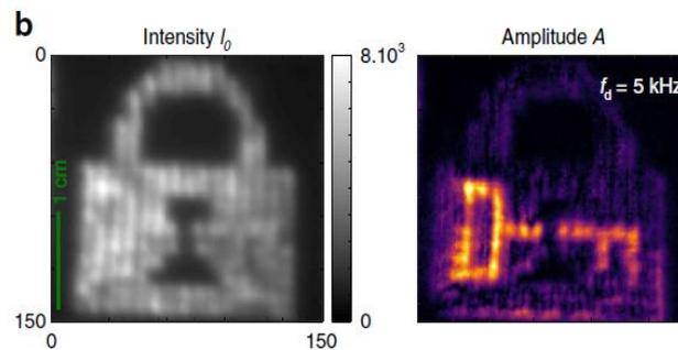
Using FAST-QUAD, the picture on the left was transmitted, which has encrypted in it the picture of a key and is not normally visible. Upon demodulation at the correct frequency, the image of the key is retrieved.
