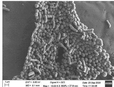
Hydrophobic Coated (Water contact angle 100°)
