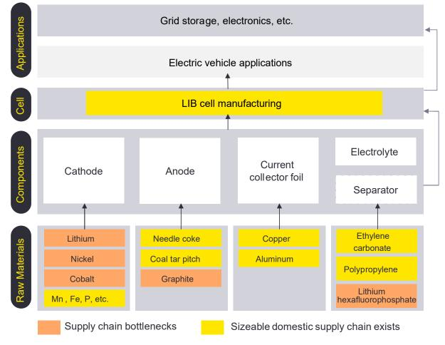
Figure 28: Key components and materials for manufacturing LIBs
