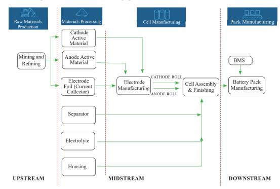
Figure 7: Sub-processes of a battery production value chain
