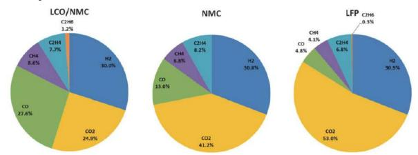
Figure 26: Effect of cathode chemistry on gases released during thermal runaway
