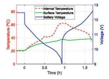
Figure 23: Internal and superficial temperature during fast charging and discharging
