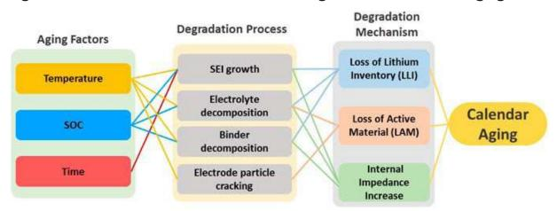
Figure 16: Overview of the factors accelerating the overall calendar aging rate
