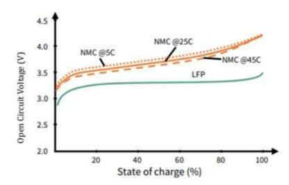
Figure 22: Open Circuit Voltage vs SoC curve of NMC and LFP cell
