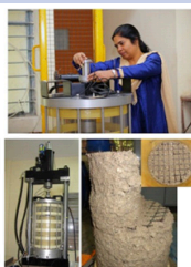
Fig. 1 Large cyclic triaxial test facility at IISc and a tested specimen of pavement material with geosynthetic reinforcement
