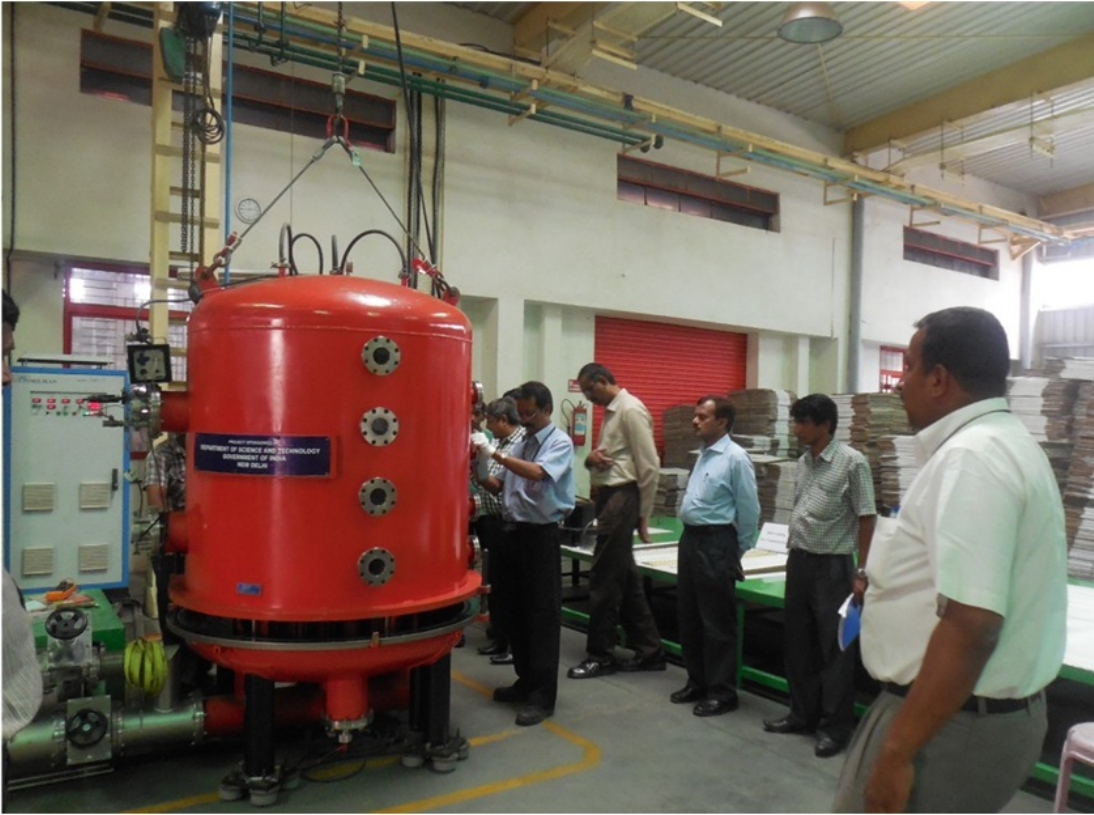
Figure 2: Plasma Treatment System to Treat Brass Valves at M/s. Triton Valves Ltd., Mysore
