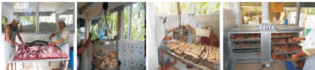
Fresh Tuna Fish cutting Tuna Loins for boiling Boiled loins for smoking Smoked loins in drayer
