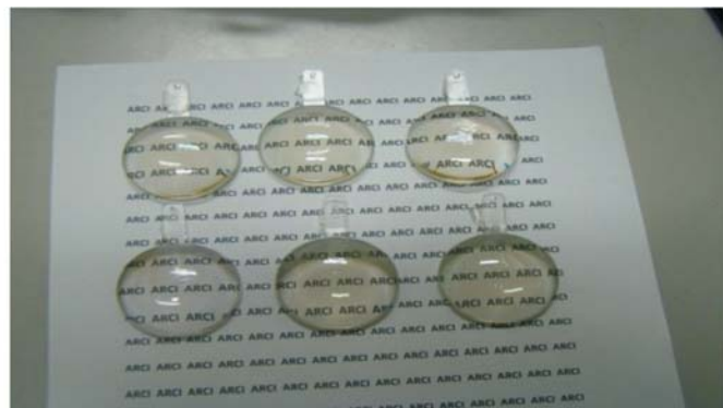
Fig. 4.52 : Sol-Gel Coated Injection Molded Bi-Aspheric
