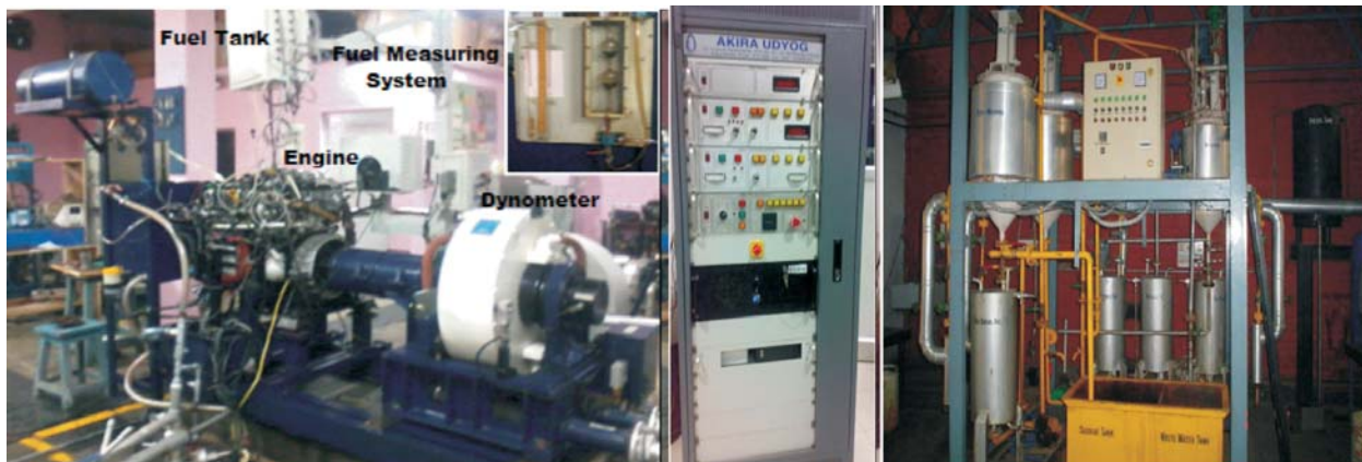
Fig. 4.38: CRDI Diesel Engine coupled with Eddy Current Dynamometer and Controller
