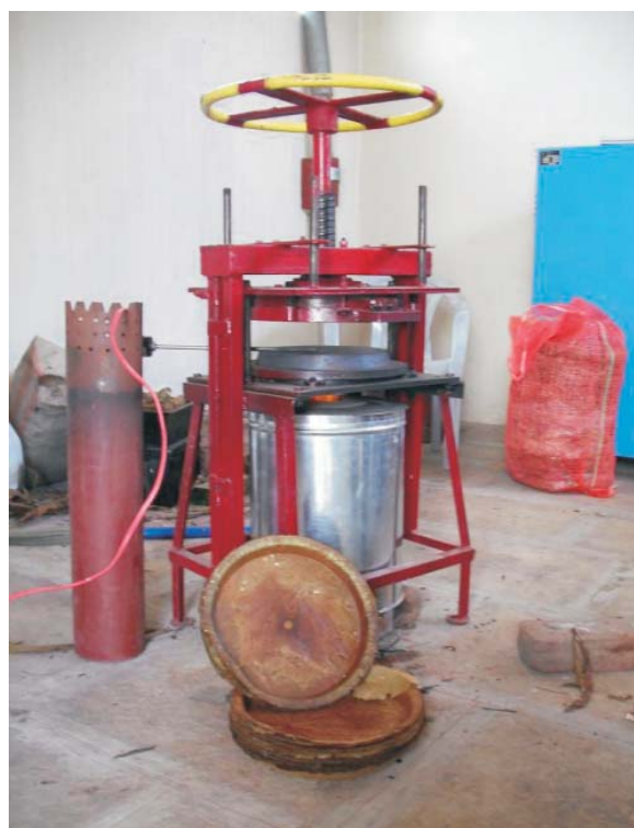
Fig. 5.7: New Design of portable fuel efficient metallic stove for making leaf plates.
