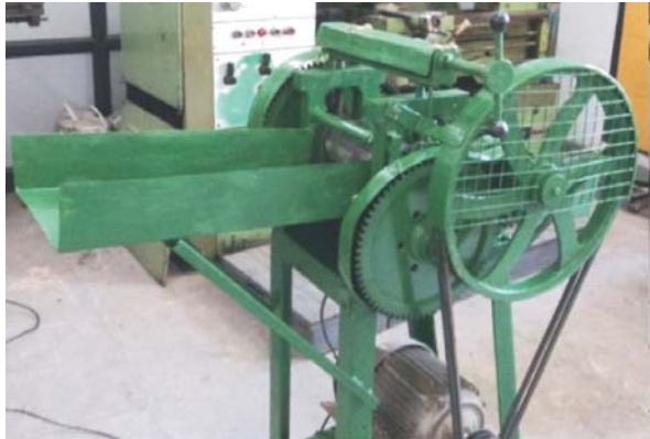
Fig. 4.62: Dewatering device for banana stem
