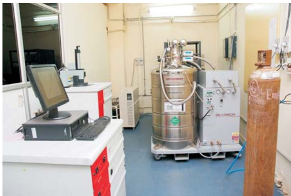
Fig. 2.1: SQUID Magnetometer with Helium mini-Liquefier at Department of Physics, IIT Madras.
