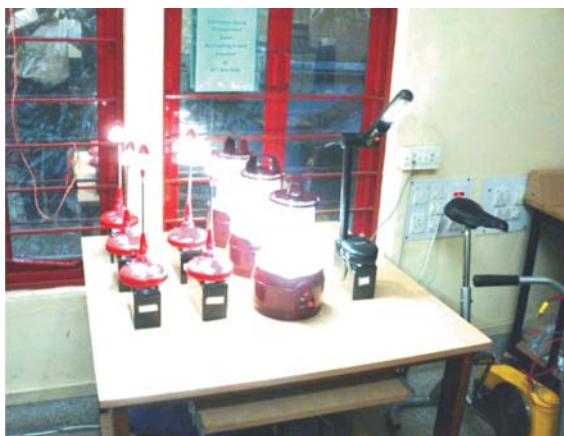
Fig. 4.59:HUC based LED lighting systems being tested
