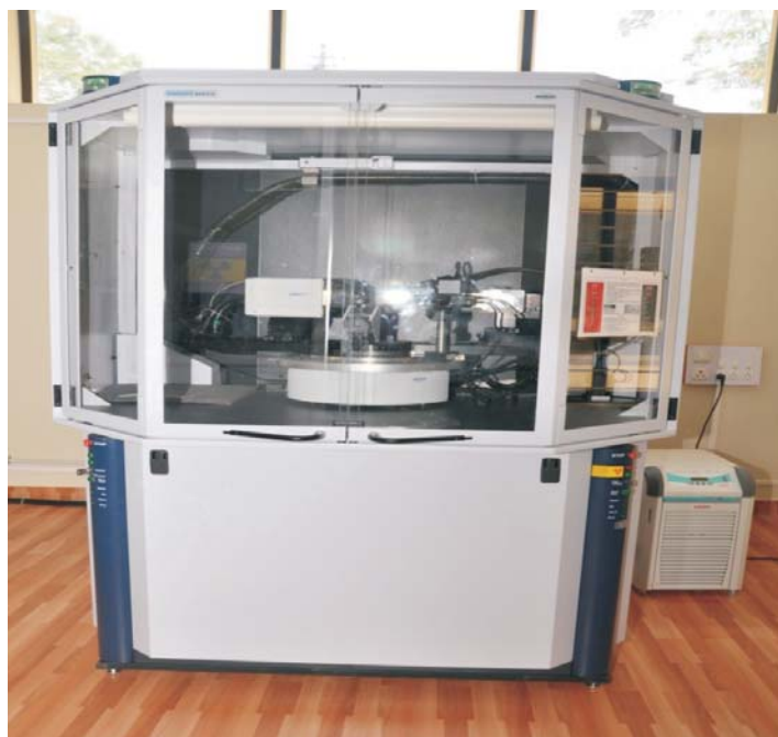
Fig. 2.5: Single Crystal X-Ray Diffractometer as a Central Facility at Karnataka University.
