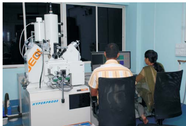
Fig. 2.2: Electron Probe Micro-Analyzer at Department of Materials Engineering, IIT Madras.
