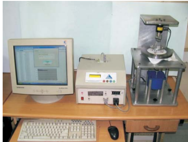
Fig. 4.13 Photograph of developed fabric friction tester
