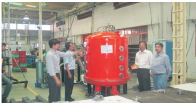
Fig. 4.40 : Industrial Scale Plasma System to treat 5000 Brass Valves per batch commissioned at M/s Triton Valves, Mysore
