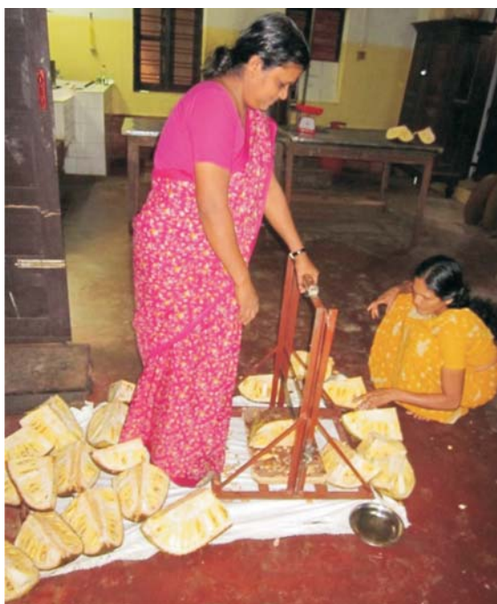
Fig. 5.2: Women workers using the Jack fruit cutter developed by Mitraniketan: Reduced drudgery with value addition
