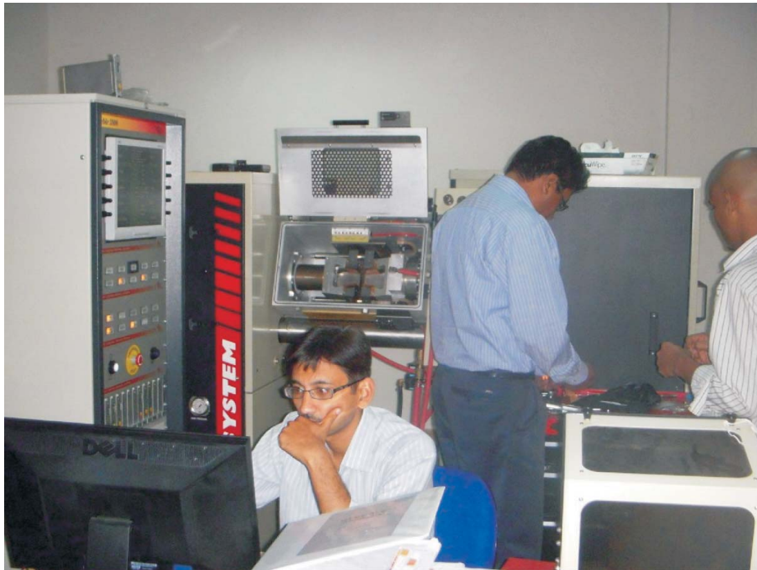
Fig. 2.3: Thermo-Mechanical Stimulator at Department of Metallurgical and Materials Engineering, IIT Roorkee.
