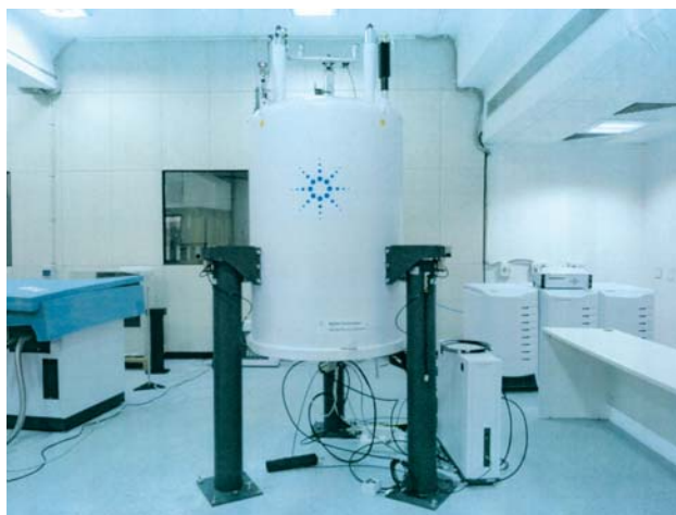
Fig. 2.7 : 700 MHz FT-NMR Spectrometer at the SAIF, Lucknow
