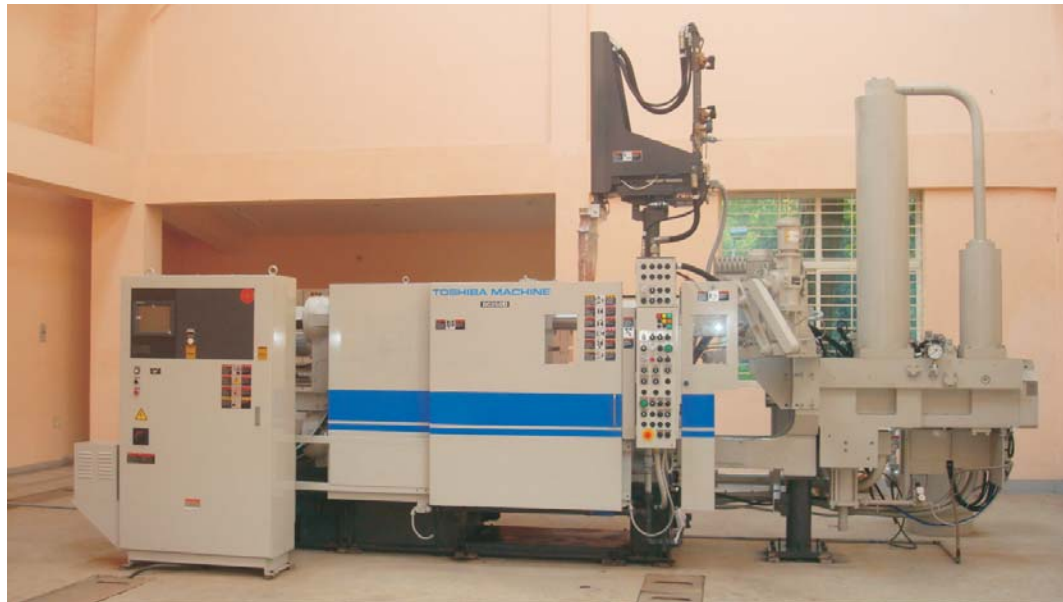
Fig. 4.67: The installed pressure die casting machine as part of the Rheo Pressure Die casting system
