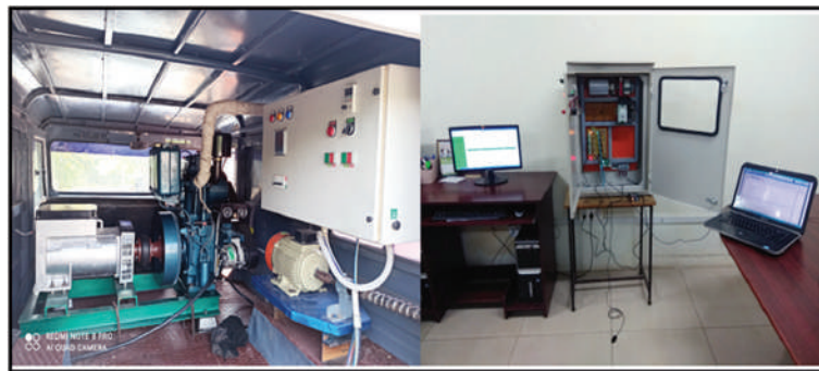
Fig. Portable Sewage Block Remover system and Control Panel
