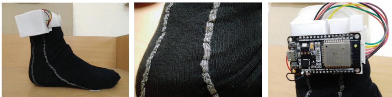
Fig. Microcontroller with Sensor embedded socks
