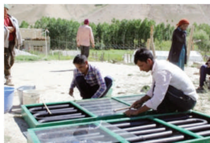
Fig. Sh. Bodh Raj and Sh Om Prakash working in fabrication activity for Solar based heating panel at Padum, Zaskar valley, Ladakh
