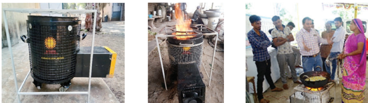
Fig. Enamel coated forced-draft improved biomass cookstove developed by SPRERI, Gujarat
