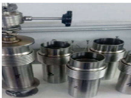
Fig. Fabrication of metal bellows expansion joints in progress (Metallic Bellows, Chennai) Prototype Metal bellows (Left), Leak test of metal bellows expansion joint in progress (Right)
