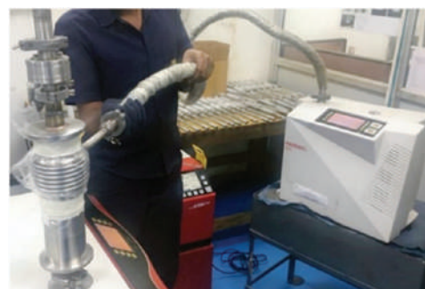
Fig. Fabrication of metal bellows expansion joints in progress (Metallic Bellows, Chennai) Prototype Metal bellows (Left), Leak test of metal bellows expansion joint in progress (Right)
